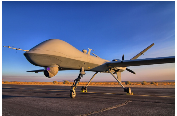
Fig. 1. The MQ-9A Reaper on the tarmac. This image highlights the physical separation between the disturbance source and the critical payload.
